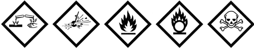
Figure 0.1 Illustration of the five symbols for dangerous substances adopted by the Council of Europe in 1962. The symbols for corrosive, explosive, inflammable, oxidizing, and poisonous substances are shown from left to right. The ILO had already proposed four of these symbols in 1952. Source: Rodgers et al., International Labour Organization , 123, fig. 3. Published with permission.
